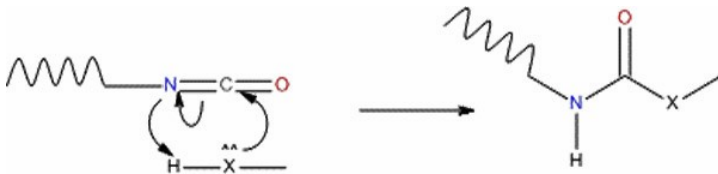
Abbildung 3: Polyurethane (X = O); Polyharnstoffe (X = NH) aus Isocyanaten
